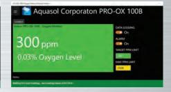
When the oxygen content reaches the operator set TARGET PPM level, the numerical value will display on a **GREEN** screen, a visual signal that welding can commence per the operator's instructions.
