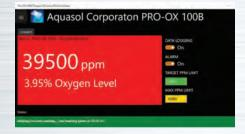
When the oxygen content reaches the operator set MAXIMUM PPM level, the numerical value will display on a **RED** screen until the oxygen level drops.
